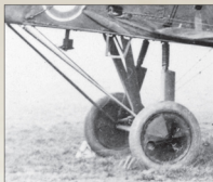
< Detail of 'Trafford Jones' undercarriage from 6934 'Punjab 26 Jullundur' with faired front struts (D33) and oleos (H24).
