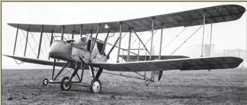
Boulton & Paul built FE.2b S203 is seen here shortly after completion in November 1915. Before being crashed and written off in October 1916 it would have the presentation name 'River Plate' applied to the side of its CDL nacelle and 'Esperanza' on the tip of its grey nose. Note the bare aluminium engine cowls, gravity petrol tank and teardrop fairing (H1) & (H2) on the undercarriage.
