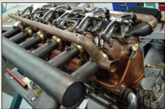
Top view showing the rocker arms, water outlet pipe and cylinder water jackets before being mounted into FE.2b 6341.
