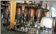
The same engine after a few hours flying time in FE.2b 6341. Note the extensive oil staining and patina of the copper water jackets and intake pipes (E24) and how necessary the protective magneto cover (B17) was.
