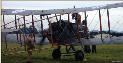
Contact! 160hp Beardmore engine #2192 roars(!) into life in April 2009.
