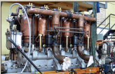
An original 160hp Beardmore engine is readied for The Vintage Aviator's FE.2b 6341 reproduction. Note the oil pump (E21) at left.
