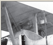
8 gal petrol tank detail from 6356 photographed after its capture on 9 March 1916. Tank is unpainted, possibly tin plated with black p brackets.
