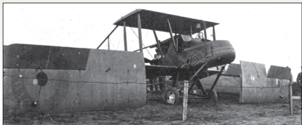
Wings removed for display. The inner tube is now safely in the possession of the German Army and half the paint from the wheel cover has worn off in the process. It is not often that the upper surfaces of wings are so clearly shown in photos. Note the painted/varnished out white areas of the cockades and the numerous CDL bullet hole patches.
