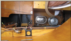
Cockpit detail from The Vintage Aviator LTD's beautiful reproduction FE.2b 6341. Note the location of the magneto winder and rudder control cable pulleys in the 'pilot's locker' layout. All following colour FE.2b photos are of this remarkable aircraft.
