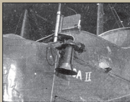
Klaxon horn used to communicate with infantry during offensives fixed to 18 Sqn FE.2b 6346 during October 1916.
