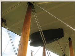
8 gal petrol tank detail from 6341 painted PC10.
