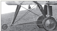
'Tricycle' oleo undercarriage with nose wheel detail from 6351 'Baroda 14'. The teardrop shaped fairing (H19 & H17) behind the front wheel is not currently fitted, note the area worn bare on the oleo undercarriage strut.
