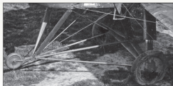
Oleo undercarriage detail from 6341 showing foot step (H8) and wind driven petrol pump (A44).
