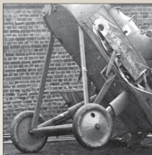
< Detail of 'Trafford Jones' undercarriage from 6934 'Punjab 26 Jullundur' with faired front struts (D33) and oleos (H24).
